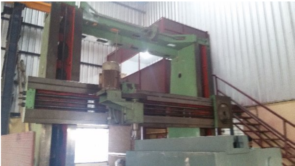
PLANO MILLING MACHINE WITH BETWEEN COLUMN SIZE OF 2.5M
